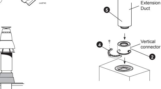
**6.** If the last extension duct requires cutting, measure 'X', the distance (outer ducts), between the duct and the terminal and add 100 mm to this dimension. This gives the length of the last extension duct.
