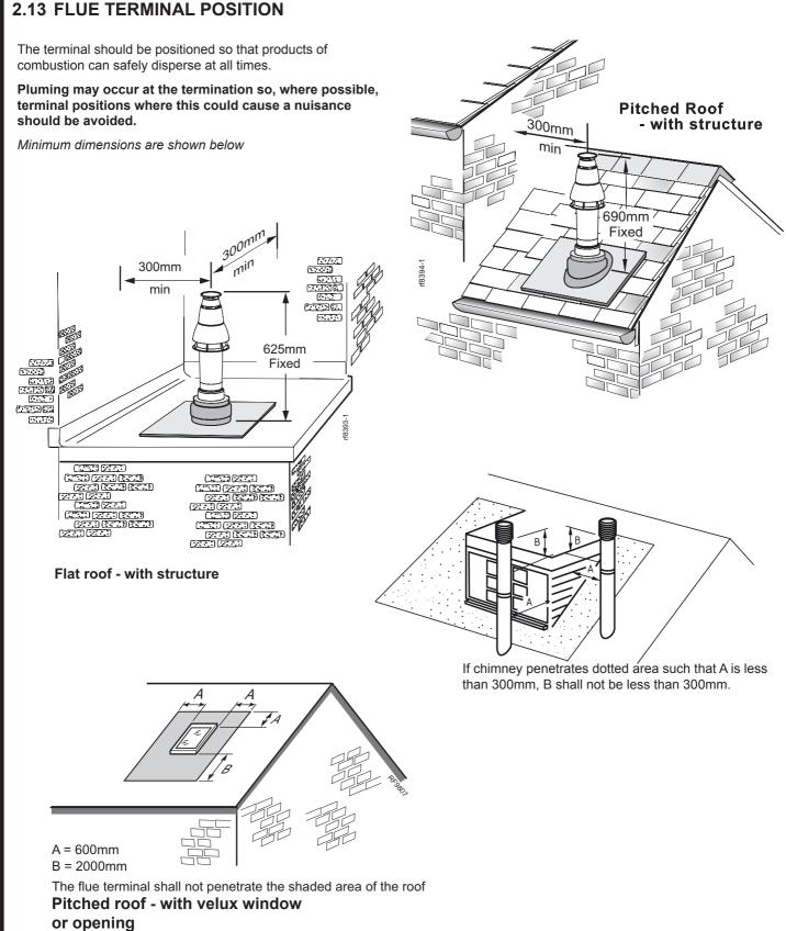
Where two or more vertical fanned draught chimney configurations terminate in close proximity at the same height, they shall be separated by at least 300mm. Where any one vertical outlet is more than 300mm above the other, then they shall be separated by at least 1500mm.
