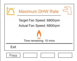
The boiler will run at Maximum DHW Rate for 10mins as long as there is sufficient cooling load
