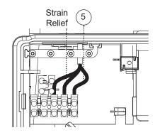
Swing the control box back up into the operating position and re-fit the front panel ensuring a good seal is made.
