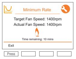
The boiler will run at Minimum Rate for 10mins
