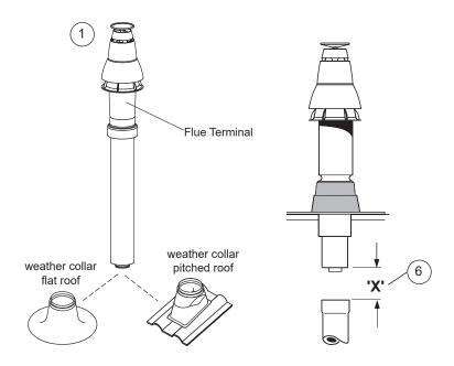
**5.** Push extension duct (if required (supplied separately)) into vertical connector.
