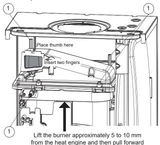
Pull the burner out from the left hand side of the boiler once it is in the vertical position.
