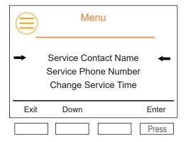
**Note.** For Diverter Valve Mid Position, press 'Down' until mid position highlighted.
