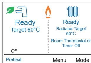
5. Check the correct operation of the timer (if fitted) and all other system controls. Operate each control separately and check that the main burner responds.
