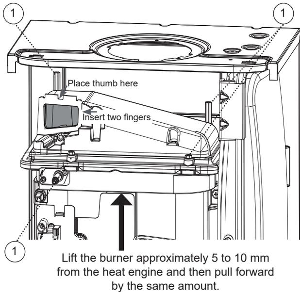
4. Pull the burner out from the left hand side of the boiler once it is in the vertical position.
