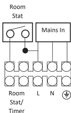
**Diagram D: OpenTherm Programmable Room Stat**
