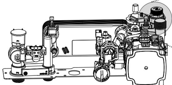
8. Check the operation of the PRV by raising the water pressure until the valve lifts. This should occur within 0.3 bar of the preset lift pressure.
