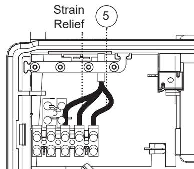
The earth connection should be longer than the current carrying connections. If the cord anchorage slips, the current carrying wires become taut before the earth.
