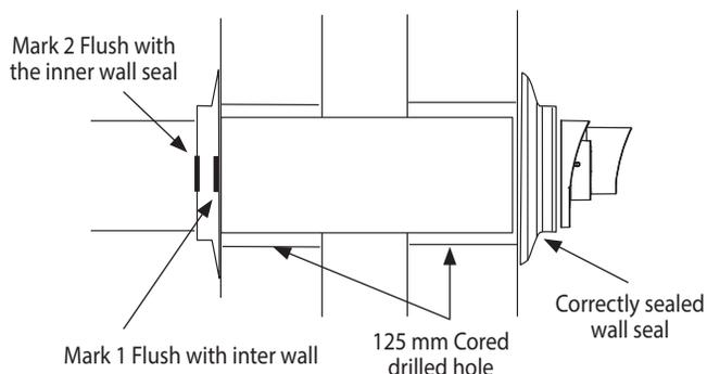
**IMPORTANT:** Ensure no White flue is visible between the flue terminal and the wall.
