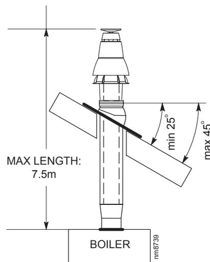
**Note.** Check the position of the inner flue duct relative to the outer duct on the assembled extension duct(s) and ensure the terminal flue duct is cut longer than the air duct to ensure engagement in the final flue duct seal.
