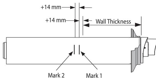
7. Place the terminal end of the flue into the 127 mm core drilled centrally and slowly apply slight pressure and move the flue up or down or side to side. This will cause the external wall seal to fold in and allow the flue to pass through the wall.
