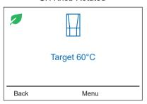
CH Knob Rotated (outside sensor connected)
