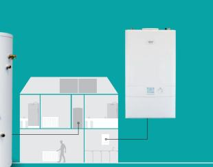
They are often thought of as a traditional boiler. They work alongside a separate hot water cylinder which is usually found in an airing cupboard, and a feed/ expansion tank often found in the loft, so they are ideal for homes that already have a heat only boiler.
