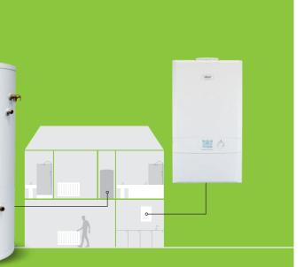
System boilers require a cylinder to store hot water, however, they don't require a feed/expansion cank, so they are ideal for arger properties with little or no loft space.
