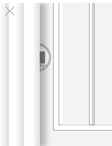
E. Not fitted behind curtains.
