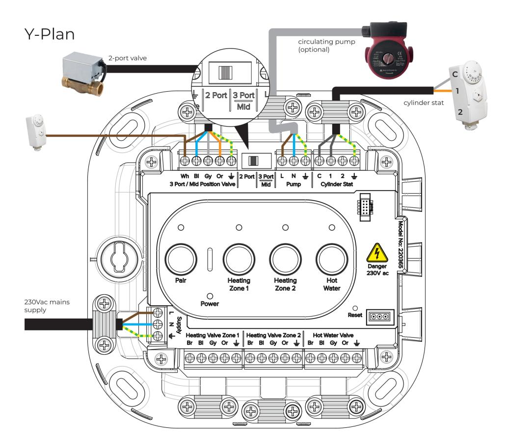
Wire the switched live from the pipe stat to the white terminal of the 3-port valve
