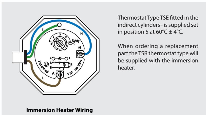
Thermostat Type TSE fitted in the indirect cylinders - is supplied set in position 5 at 60°C ± 4°C.
