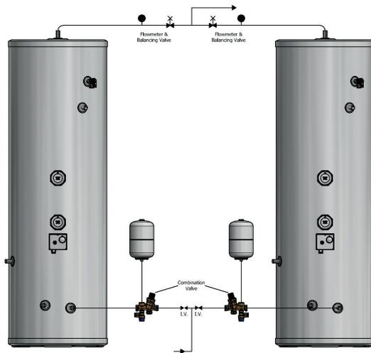
If two Ideal Pro cylinders are coupled together the secondary inlet and outlet pipes must be balanced. The units must be fitted on the same level.
