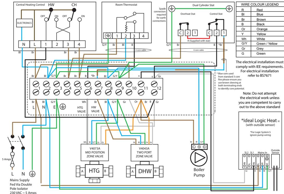
Ideal schematic wiring diagram for an inverted installation
