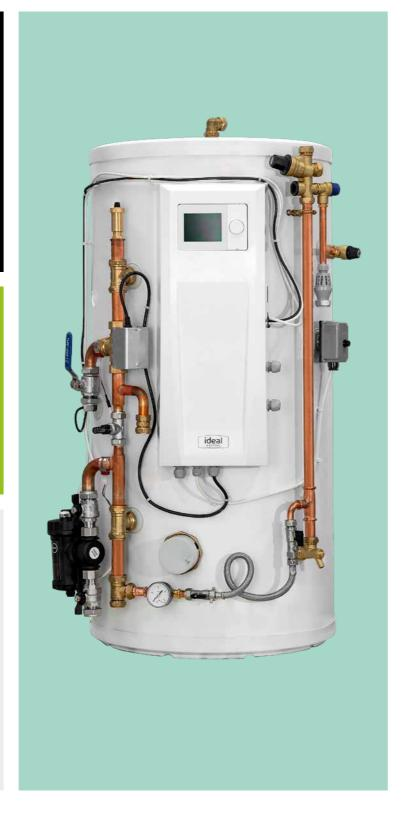
The two zone pre-plumbed cylinders include a lowloss header pre-plumbed onto the cylinder, decoupling the heating system from the heat pump, ensuring optimal flow and two zone control.
