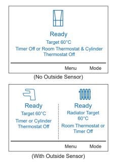
4. Check the correct operation of the timer (if fitted) and all other system controls. Operate each control separately and check that the main burner responds.
