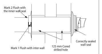
(!) **IMPORTANT:** Ensure no White flue is visible between the flue terminal and the wall.
