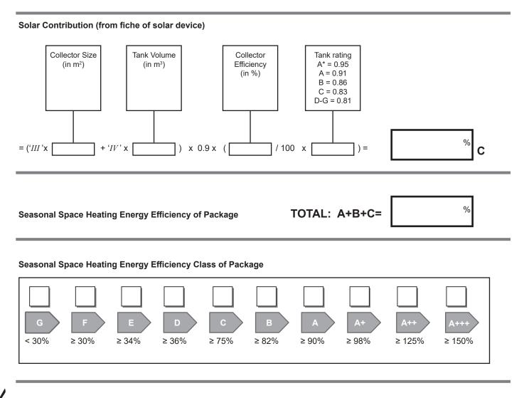
The energy efficiency of the package of products provided for in this document may not correspond to its actual energy efficiency once installed in a building, as the efficiency is influenced by further factors such as heat loss in the products in relation to the building size and its characteristics
