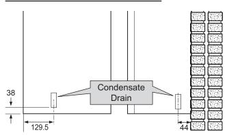
This appliance is fitted with a siphonic 75 mm condensate trap system that requires filling before operating the appliance for the 1st time or after maintenance.
