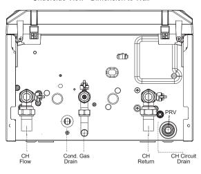
(!) **IMPORTANT:** Please ensure there is sufficient clearance either side and below the boiler, particularly from door hinges and the base of a cupboard, to allow the door to be opened to allow the pressure gauge to be checked.
