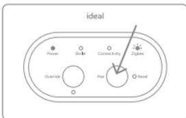
11. **Press and hold** the Pair button on the Smart Interface until the Zigbee LED starts flashing red to begin the pairing process with the Halo.
