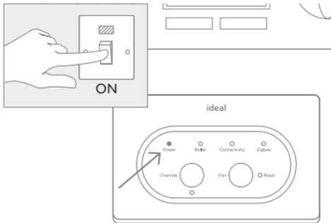
9. Switch on the boiler, the Halo Smart Interface will power up and begin setup, this can take up to 90 seconds. Once setup is complete the green Power LED should be the only LED illuminated.
