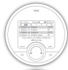
Turn the dial to move between the different days and view the schedule that is set. To edit a day, push the dial or right hand button when the day is highlighted in light blue.
