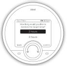
Turn the dial to select how long you would like to extend your heating for. Push the dial or press the right button to confirm your selection.
