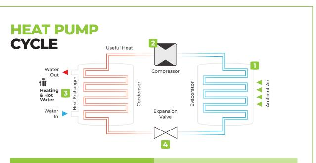
**1. Capture:** The fan passes ambient air over extremely cold liquid refrigerant. The refrigerant captures the heat from the ambient air and becomes a warm vapour.
