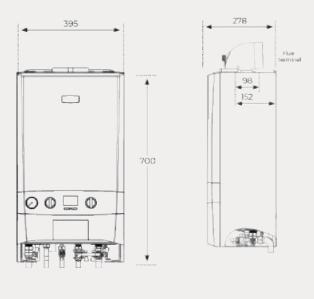
Note: The minimum front clearance when built into a cupboard is 5mm from the cupboard door but 450mm overall clearance with the cupboard door open is required for servicing.
