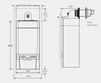
**Note:** The minimum front clearance when built into a cupboard is 5mm from the cupboard door but 450mm overall clearance with the cupboard door open is required for servicing.
