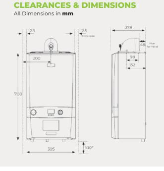
Note: The minimum front clearance when built into a cupboard is 5mm from the cupboard door but 450mm overall clearance with the cupboard door open is required for servicing.
