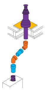
**ROOF FLUE SYSTEM WITH 2 X 45° BEND**
