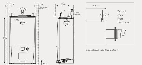
Note: The minimum front clearance when built into a cupboard is 5mm from the cupboard door but 450mm overall clearance with the cupboard door open is required for servicing.
