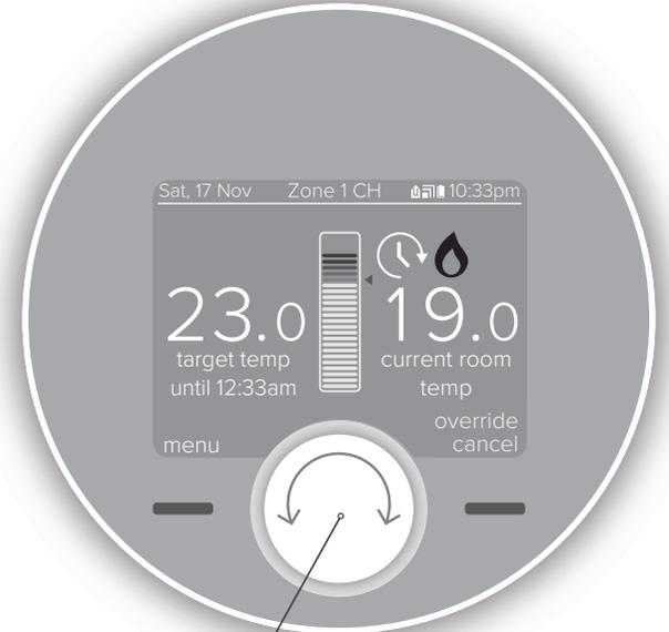
Turn the dial to adjust the target temperature temporarily (this could be up or down)
