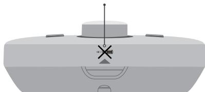
Remove all the old batteries and replace with 4 new AA Alkaline batteries. Check you have the correct battery orientation then position the Halo back onto the rear housing and gently push into place until you feel a positive click.
