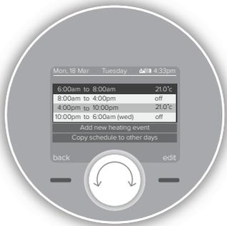
Push the dial to edit a heating time or temperature when it is highlighted in light blue. You can also add an additional heating period by scrolling and pushing on the “Add new heating event” bar. You can have up to 6 heating events per day in your schedule.
