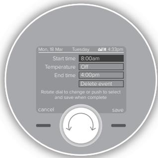
Alter the start and end times of the heating period and the temperature by scrolling and then pushing the dial to edit. Then use the dial to alter the time or temperature and push to confirm. Push the dial or the right hand button to save your changes.
