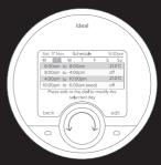
Turn the dial to move between the different days and view the schedule that is set. To edit a day, push the dial or right hand button when the day is highlighted in light blue.
