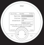
Alter the start and end times of the heating period and the temperature by scrolling and then pushing the dial to edit. Then use the dial to alter the time or temperature and push to confirm. Push the dial or the right hand button to save your changes.
