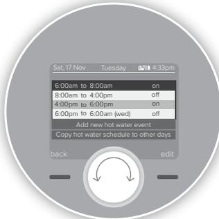
Push the dial to edit a hot water time when it is highlighted in light blue. You can also add an additional hot water period by scrolling and pushing on the "Add new hot water event" bar. You can have up to 6 hot water events per day in your schedule.
