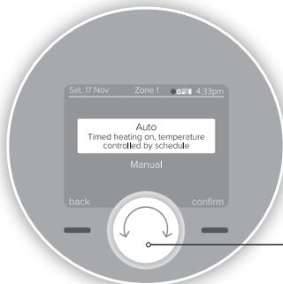
Use the dial to scroll between the different modes (Auto, Manual and Off) and then push the dial or press the right hand button to confirm your selection
