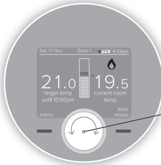
Press and hold the dial to extend the current heating setting
