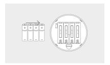
Insert the 4 AA batteries provided into the front housing of the Halo. Pay close attention that the orientation of the batteries is as indicated in the housing.
