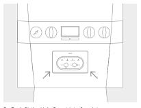
8. Push fit the Halo Smart Interface into the boiler aperture.
