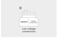
4. If an existing Opentherm device has been used, ensure its removal and add the link wire into the "opentherm" connection (see diagram) On brand new boilers the link should already be in place
