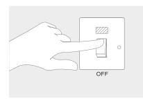
1. Isolate mains supply to boiler.
