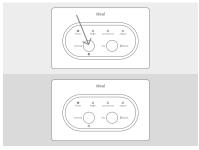
10. Check the Smart Interface connection to the boiler by pressing the Override button. The Override LED should be green and the boiler will fire. Press the Override button again to switch off the boiler, the Override LED should now go out.
