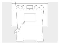
Locate the blanking plate on the front of the boiler and remove carefully with a small flat bladed screwdriver
