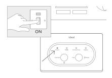
Switch on the boiler, the Halo Smart Interface will power up and begin setup, this can take up to 90 seconds. Once setup is complete the green Power LED should be the only LED illuminated.
