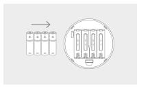
Insert the 4 AA batteries provided into the front housing of the Halo. Pay close attention that the orientation of the batteries is as indicated in the housing.
