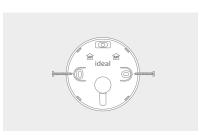
If no trim plate is required, use the rear housing of the Halo to position the unit on the wall, alternatively secure rear housing to trim plate. Take care not to overtighten the screws.
