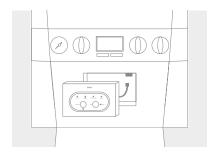
7. Connect the plug on the Halo Smart Interface to the connector in the aperture.
