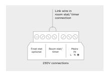
3. If existing 230V device is already installed remove wiring from the 230V connections and add the link wire into the room stat/timer connection (see diagram). On brand new boilers the link will already be in this position.
