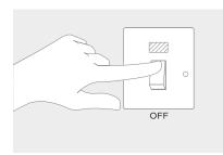
1. Isolate mains supply to boiler.
