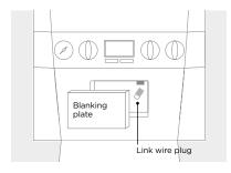
Remove link wire plug and keep in a safe place.
