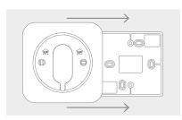
The Halo can be installed with or without the provided trim plate.
