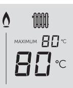
**Boiler is active for Central Heating**
