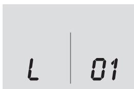
**Boiler is in Lockout for a specific error.** Display will show a number after the "L" to indicate which error is detected
