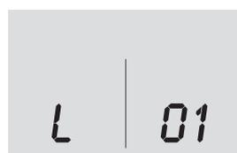
**Boiler is in Lockout for a specific error.** Display will show a number after the "L" to indicate which error is detected
