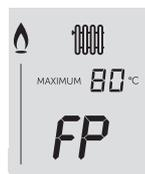
**Boiler is active for boiler frost protection:** operates if the ambient temperature is below 5°C until it reaches 19°C.
