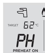
**Boiler is heating up the Plate Heat Exchanger**
