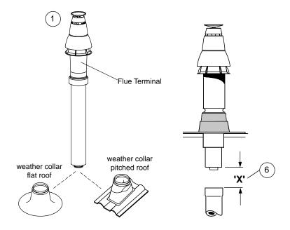
Push extension duct (if required (supplied separately)) into vertical connector.
