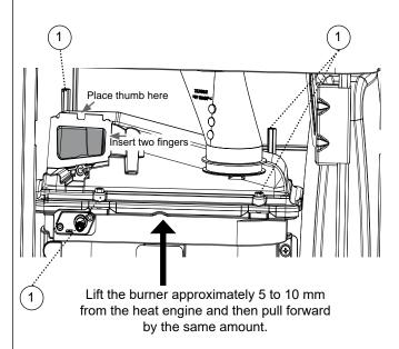
4. Pull the burner out from the left hand side of the boiler once it is in the vertical position.
