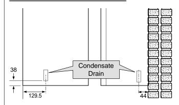
This appliance is fitted with a siphonic 75 mm condensate trap system that requires filling before operating the appliance for the 1st time or after maintenance.
