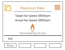
The boiler will run at Maximum Rate for 10mins as long as there is sufficient cooling load
